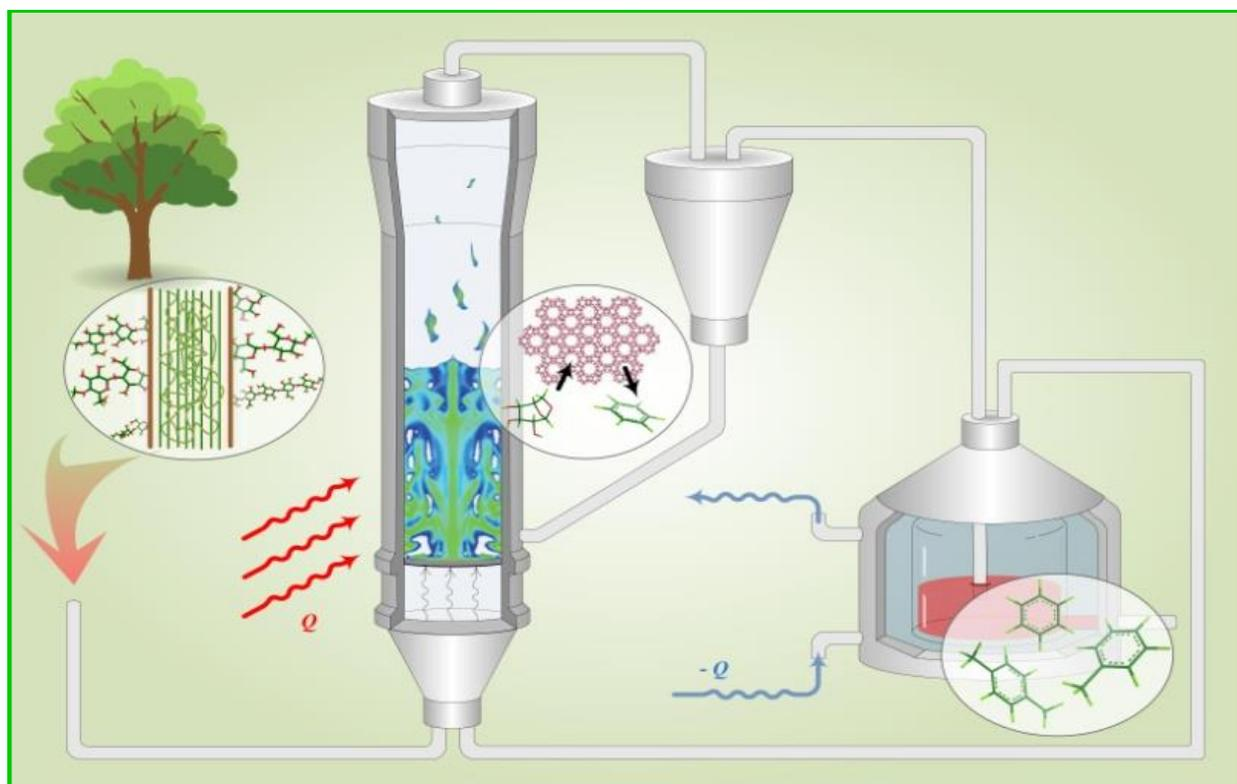
Schematic of catalytic fast pyrolysis.
